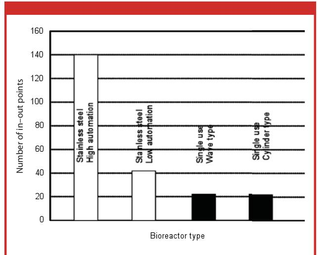
**Figure 3:** Comparison of the number of in-out points in various bioreactor systems (1).
