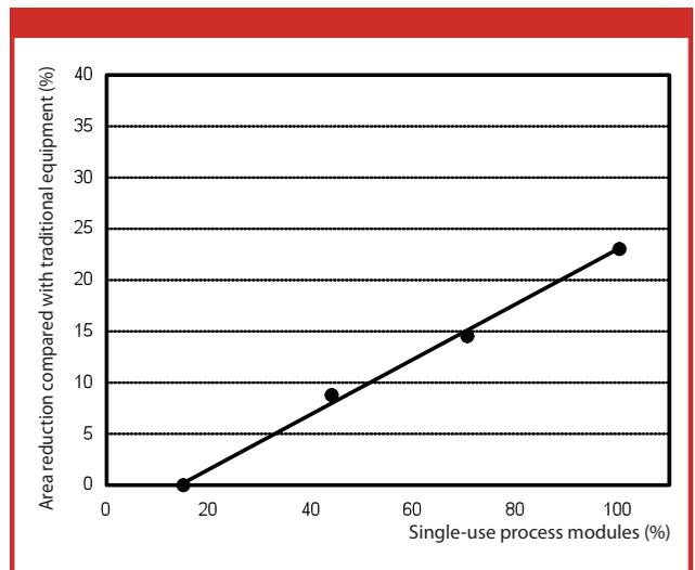
**Figure 2:** Reductions in process-room area associated with various degrees of single-use equipment installation in an upstream biopharmaceutical process (1).
