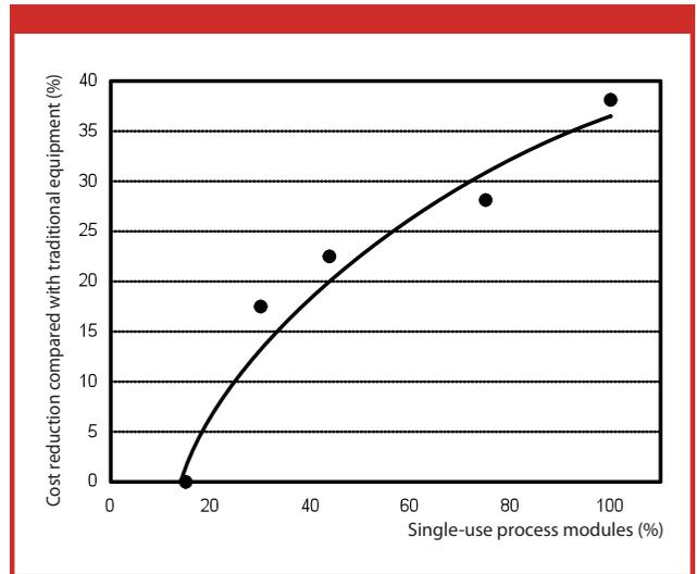
**Figure 1:** Reductions in investment costs associated with various degrees of single-use component installation in an upstream biopharmaceutical process. Simple single-use technology generally represents a smaller cost than does traditional equipment (1).
